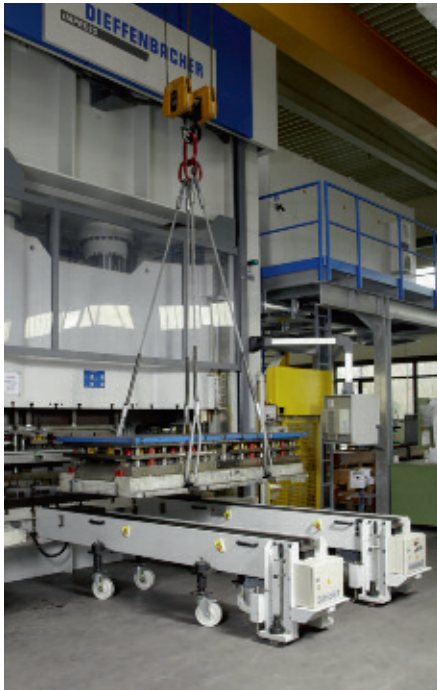
Die loading arms with spring-mounted transport rollers
