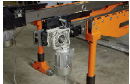
Parallel die displacement using an "electric" shaft
