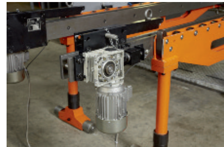
Parallel die displacement using an "electric" shaft
