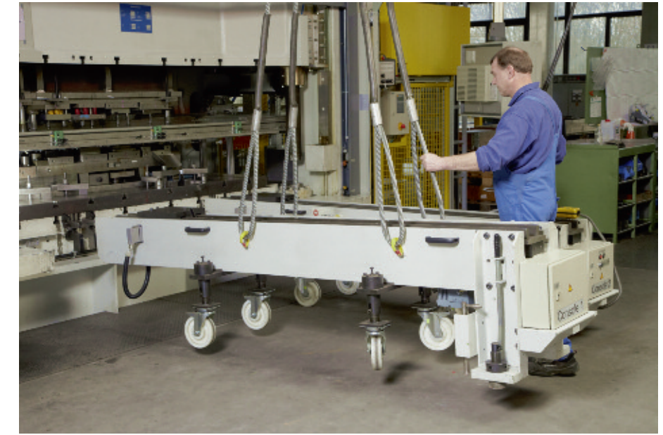
Transportation of die loading arms by an overhead crane or mobile support legs
