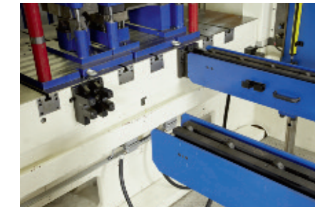
Die loading hooks with a safe locking mechanism
