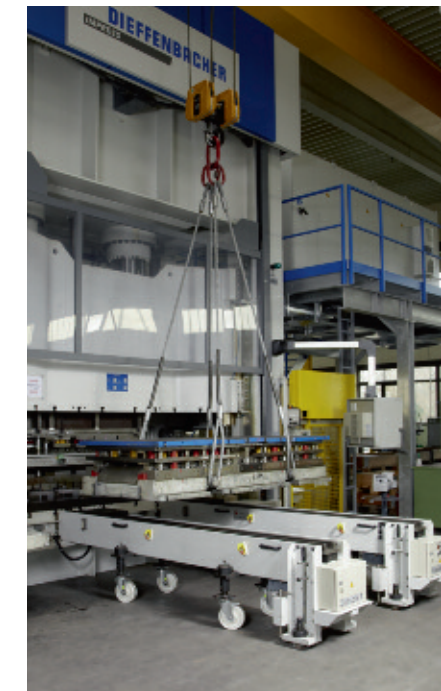
Die loading arms with spring-mounted transport rollers
