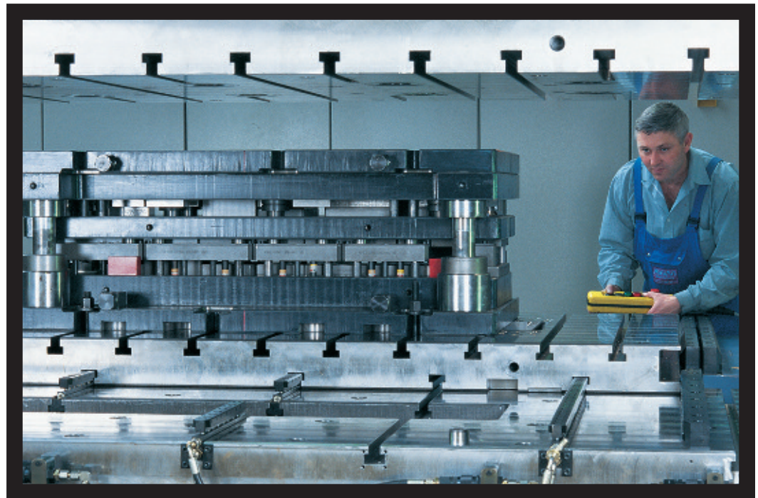
Subplate technology. Press table equipped with DILOS SlipGrip SGR28H, press ram equipped with DILOS Swing Sink Clamp
